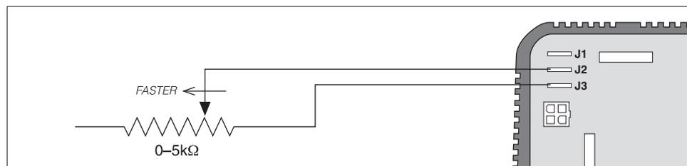
Mechanical potboxes and footpedals are Type 0 throttles. It doesn't matter which wire goes on which terminal, and the wires can be extended as required.
