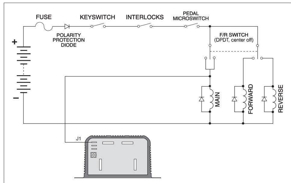
Wiring for mechanical reversing switch (golf car type)
