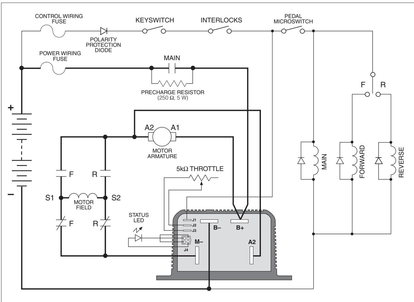
**Fig. 3** Basic wiring diagram, Curtis 1204M/05M motor controller.
